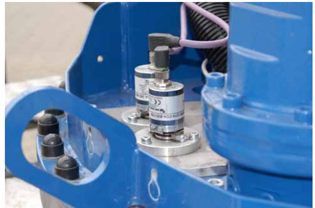
Image 4 WDGA absolute encoders from Wachendorff record the rotation of the boom on its own axis. For safety reasons, the entire safety system is designed with redundant sensors and controls – this is why there are two encoders side by side, each working completely independently. Thanks to EnDra@multiturn technology, the encoders are non-wearing and work without a battery.
